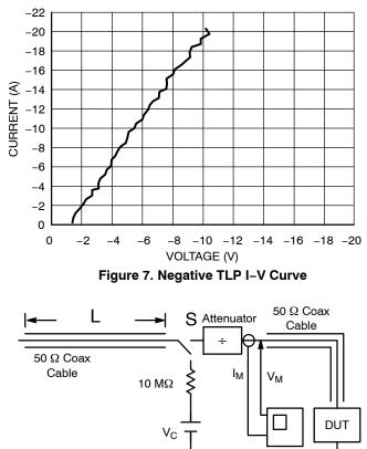
Figure 8. Simplified Schematic of a Typical TLP System
