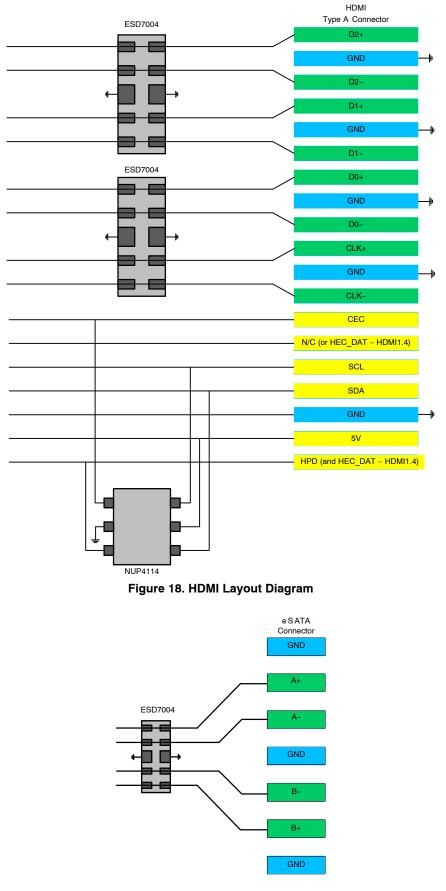
Figure 19. eSATA Layout Diagram
