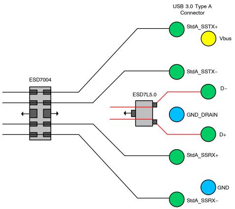
Figure 16. USB3.0 Standard A Connector Layout Diagram
